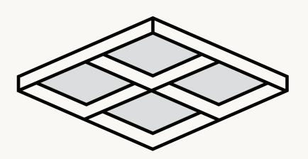
Framework 'Capped' design is a full coverage system with a large surface area; ideal for concealing ductwork, cabling and other ceiling fixtures, while offering superior acoustic performance.
