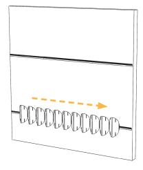
7. Secure next row above by connecting slots in the tiles. Friction alone will hold the tiles in place.
