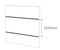
3. Cut Z clip to length of wall and secure at 300mm centres. **Note:** On concrete wall, please use wall plugs. On wood or steel wall, self tapping screws can be used.
