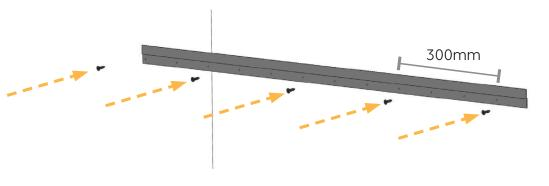
4. Subsequent rails to be mounted 1070mm apart. This is crucial for the tiles to align correctly.
