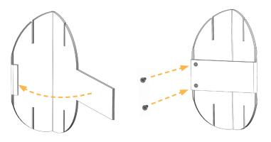
2. Secure Z-clip only to rear of all tiles that secure to Z-Clip wall rail. Align top of clip with top of flap. Tiles that do not attach to the wall rail do not require Z- clips on rear.
