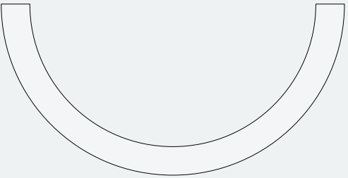
Swing Profile Hight - 305, 457 or 610mm Width - 610, 915 or 1220mm Depths - 102mm
