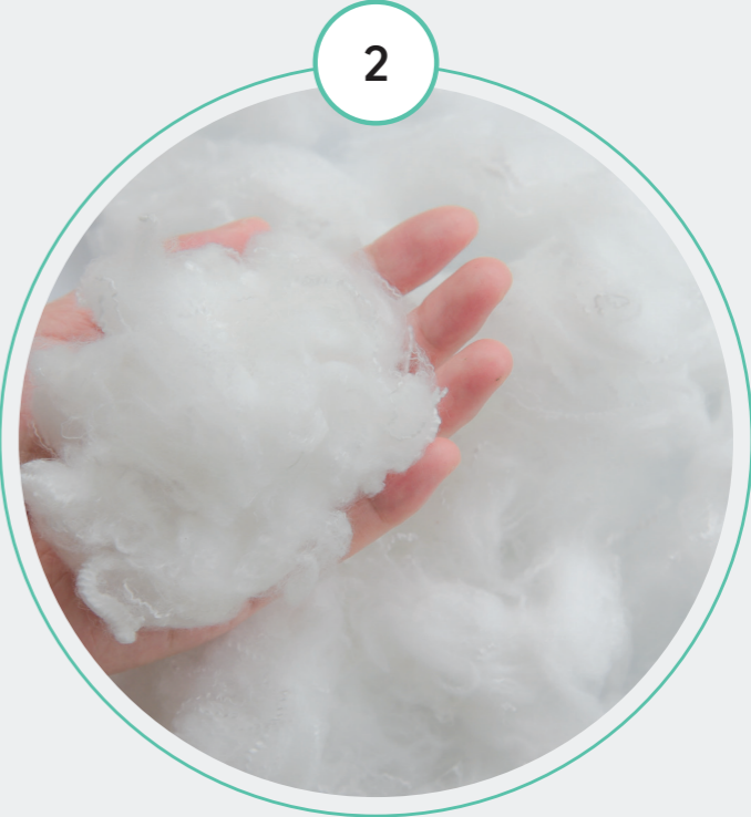
The discarded drink bottles are cleaned and cut into flakes before being melted and extruded into fibers of natural white color.
