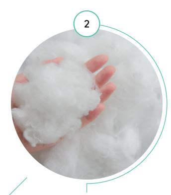
The discarded drink bottles are cleaned and cut into flakes before being melted and extruded into fibers of natural white color.
