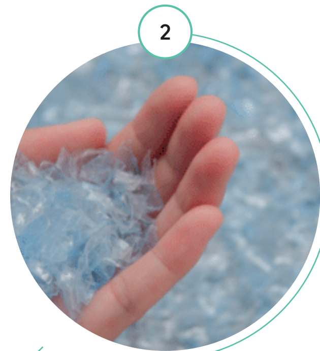
2 The discarded drink bottles are cleaned and cut into flakes before being melted and extruded into fibers of natural white color.
